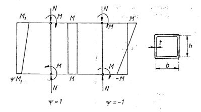
Fig.1 Bending moment distributions on a SHS beam-column
