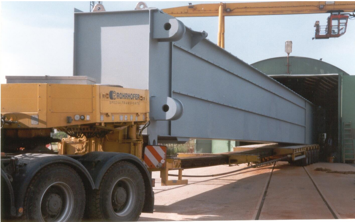
Fig. 3. Transportation of the welded box-beam
