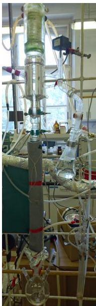
Figure 2 Laboratory column for COD-reduction of PWW
