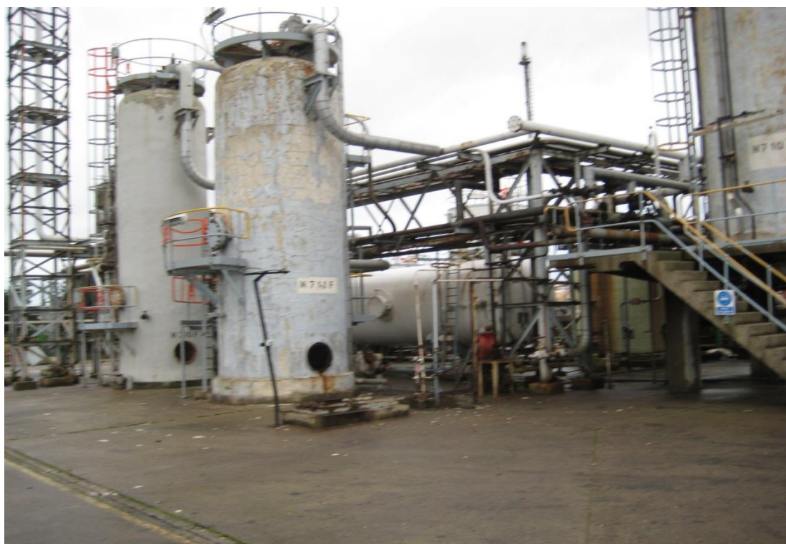
A part of 7500 BPD MEROX TM unit to remove mercaptan sulphur from kerosene fraction offered for sale by Phoenix Equipment Corp ( https://www.phxequip.com/plant.2204/merox-unit-7500-bpd.aspx )
