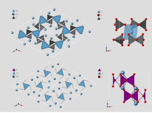
Two structural model of HAp-CAp end-members. CAp's model based on the finnemanite (Pb<sub>5</sub>(AsO<sub>3</sub>)<sub>3</sub>Cl; Baikie et. al 2008) structure.
