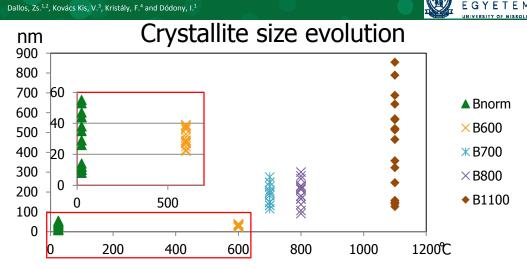
Heating experiment Organic matter Lath-like crystals, with 5 nm maximum length Spherical crystals, with 40 nm diameter Euhedral crystals, with 100 nm maximum length Euhedral crystals, with 150 nm maximum length Euhedral crystals, with 500 nm naximum ength 800 °C 700 °C. 2° 000 600 °C 1000 °C 1100 °C
