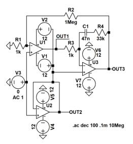
Fig.3. LTSpice simulation model for high CMRR composite amplifier in Fig.2.
