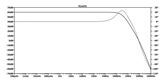
Fig.4. Gain and phase characteristics of the composite amplifier in Fig.2.
