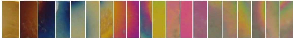
Figure 3 Sections of surfaces of the anodising nanograin Grade 2 titanium discs, with voltage changing from left to right from 10 to 200 V in 10 V increments
