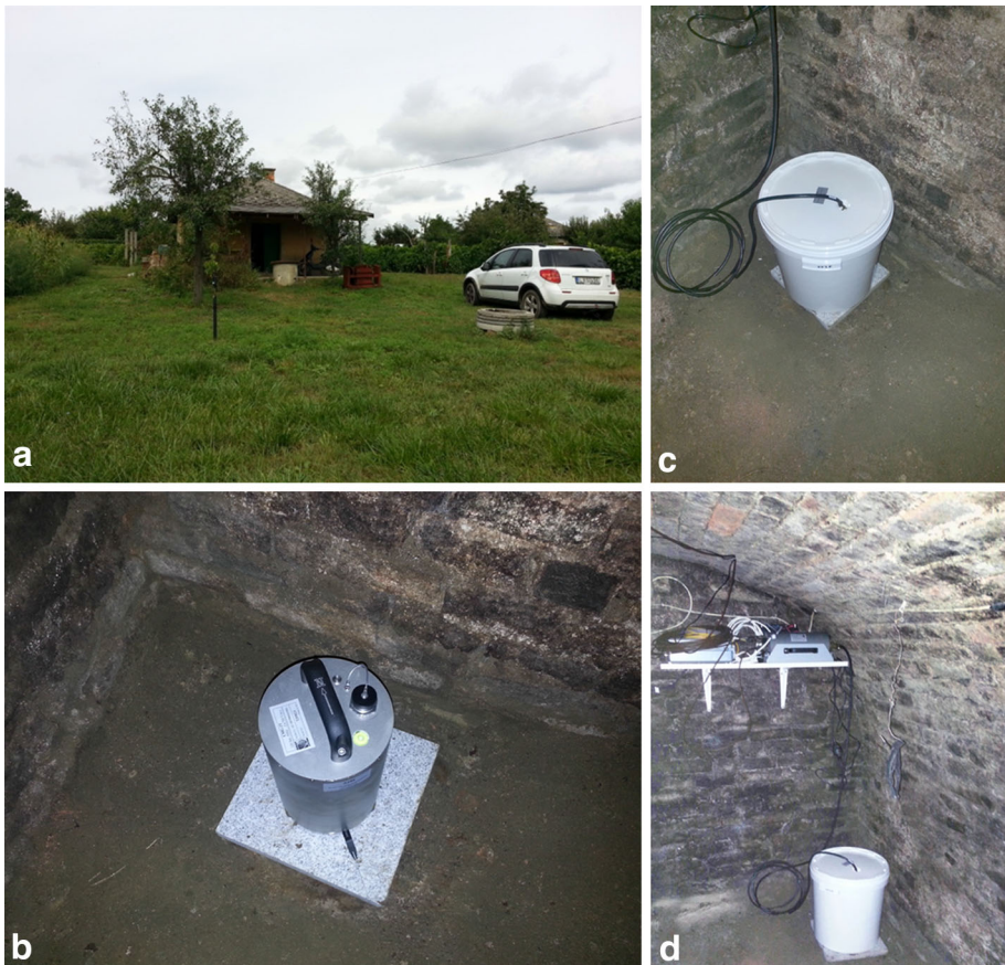
Fig. 2 A typical station configuration for the AlpArray project. a The selected one-storey building for station A267A. b Sensor after levelling and orientation with magnetic compass. North direction is marked on the granite slab. c For thermal insulation the sensor is covered with a pail filled with polystyrene packing foam peanuts. d The installed station. GPS antenna is mounted through the vent chimney. (Color figure online)
