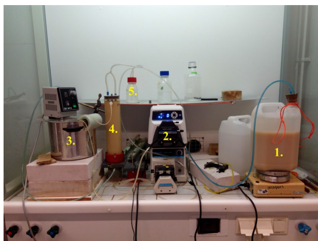
Fig. 3 The experimental apparatus with gas-permeable hydrophobic membrane
