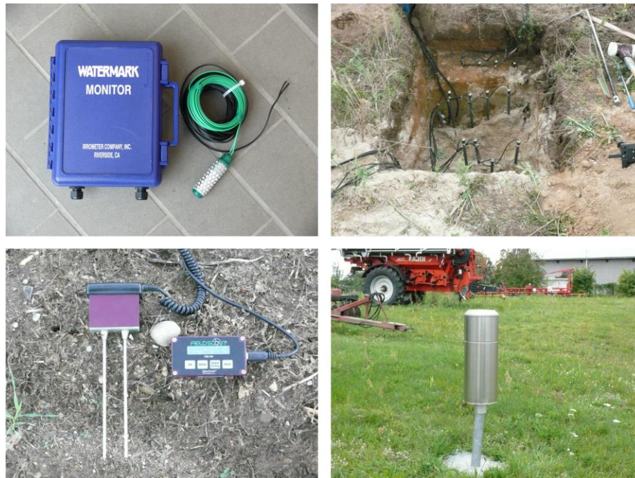
Figure 4. Essential measuring instruments used at the pedo-hydrological monitoring places in Flaeming; top left: Watermark sensor with data logger; top right: redox sensors; bottom left: mobile TDR-sensor; bottom right: rain gauge.
