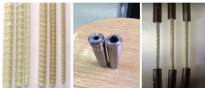
Fig. 1. GFRP bars and their examination
