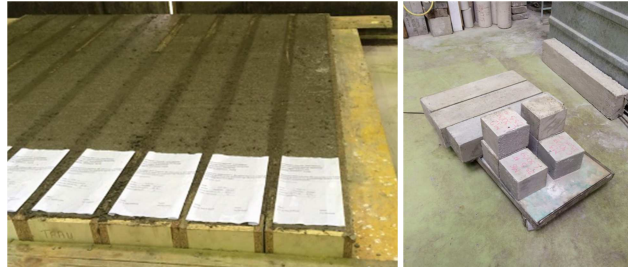
Fig. 3. Set of concrete beams and concrete cubes for examination
