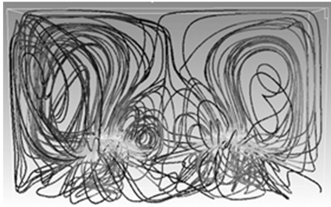
Fig. 2. Streamlines starting from mixer plane (rpm: 100 and 400 \text{min}^{-1} )
