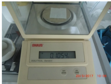
Fig. 8. Weighing of the suction fleece used to dab specimen of plaster surface
