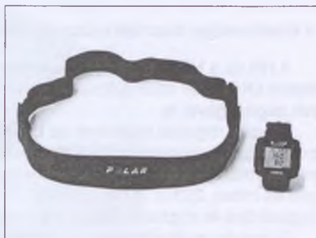
Photograph 3. Polar HR transmitter with elastic belt and Polar HR monitor (Hagen et al., 2005)
