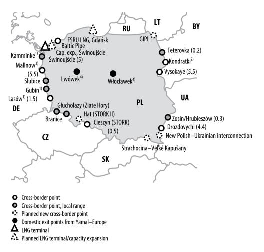
Figure 2. Cross-border pipeline gas and LNG import capacity into Poland
