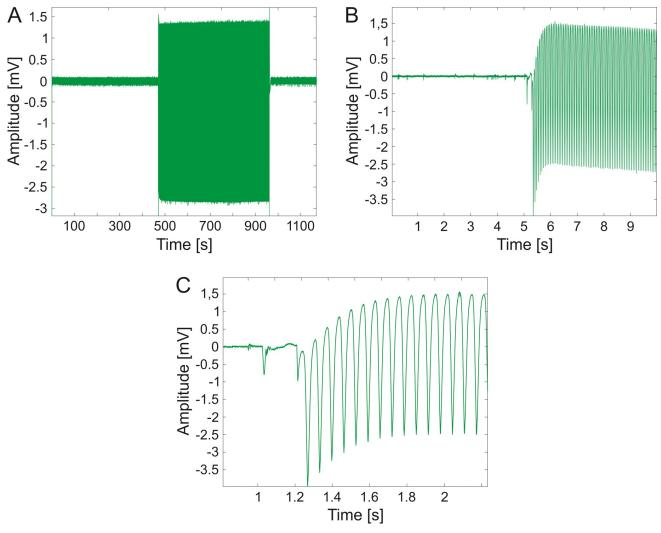
**Fig 2. Representative sample of the imaging laser impact on the electrophysiological recordings.** Between the first and the last parts of the measurement, which were recorded without two-photon imaging, photoelectric artefacts of the two-photon imaging laser are observable (A). The recorded data at the moment when the imaging laser was switched on (B, C).
