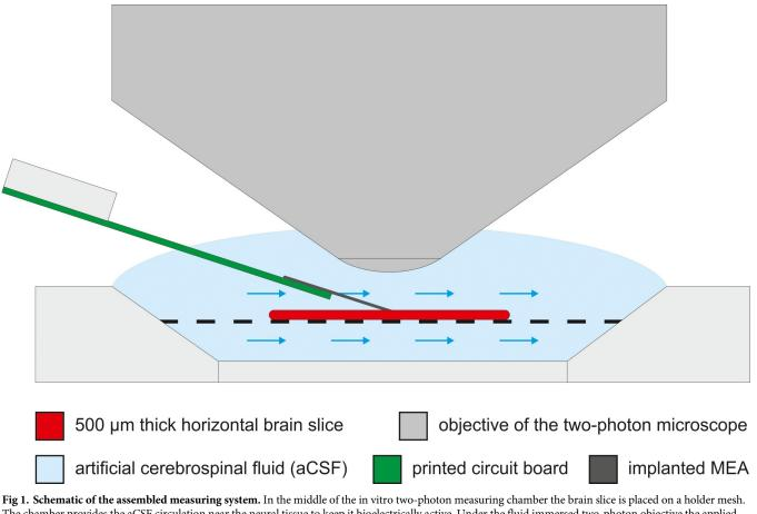
The chamber provides the aCSF circulation near the neural tissue to keep it bioelectrically active. Under the fluid immersed two-photon objective the applied MEA was inserted into the tissue.
