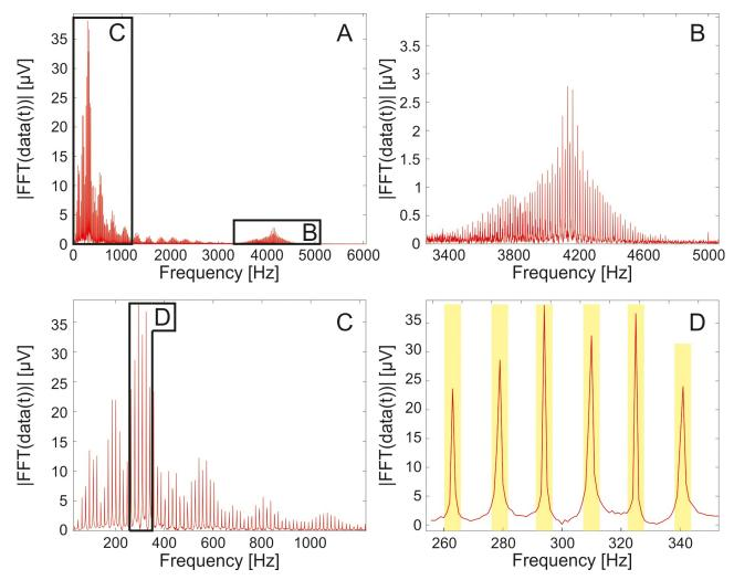
**Fig 4. The absolute value of the frequency spectrum of the electrophysiological recordings.** The fast Fourier transform analysis of the imaging laser generated noise in the electrophysiological recorded data (A). Harmonics below 1200 Hz (C) and at higher frequencies (B) of the laser generated periodical artefacts appeared with high magnitudes. The overlap of the harmonics is observable (B). A part of the rejected frequencies by the custom-set comb filter is shown in yellow (D).
