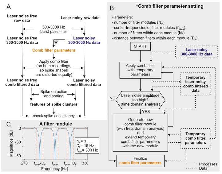
Fig 3. Filtering and analyzing steps. The performed filtering and analyzing steps in order to identify the spike clusters and check the spike consistency between the two-photon imaging laser noise free and the laser noisy data (A), the parameter setting algorithm of the applied custom-set comb filter (B) and the result of the parameter setting of a representative filter module (C).
