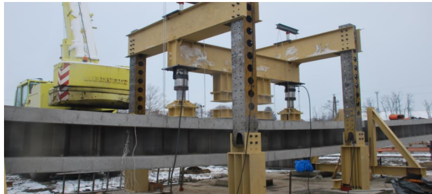
Fig. 4. Full scale test of the developed hybrid bridge girder with corrugated web.
