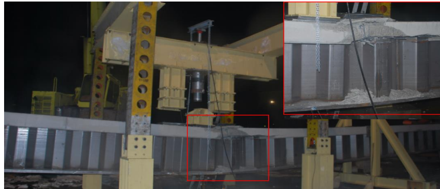
Fig. 3. Full scale test of the developed composite bridge girder with corrugated web.
