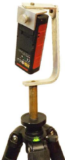
Figure 8 – Tripod Head for DistoX2
