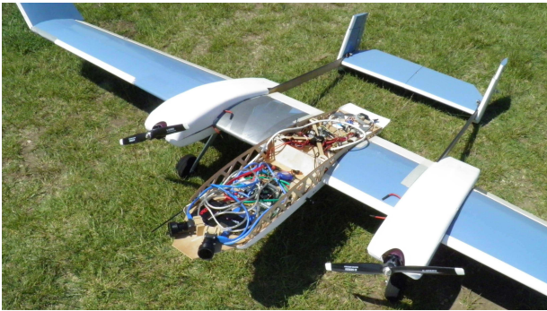
Fig. 4. Sindy 3.5m wingspan, 12kg own aircraft
