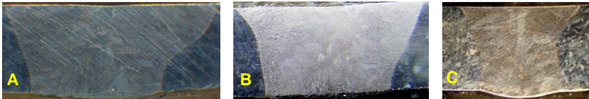
Figure 14. Cross section of characteristic weld beads: (A) TIG with 100 % Ar, (B) TIG with 70 % Ar + 30 % He shielding gas and (C) ATIG welding on 3 mm thick plates. Note the differences between the bead widths.
