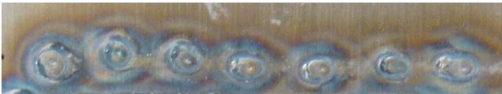
Figure 7. The surface of a 2mm thick plate welded with 40 Amps; note the arc restriking points.
