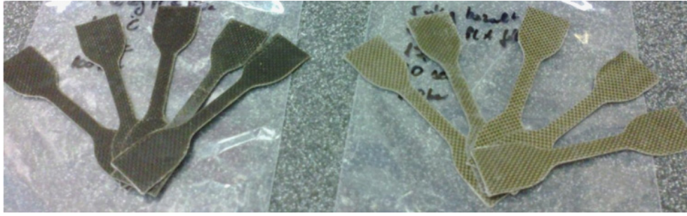
Figure 4. Test specimens produced at 220°C (left) and at 190°C (right) by using 300 bar pressure
