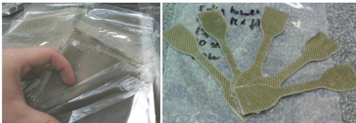
Figure 1. Film-stacking process (left) and the final basalt fabric reinforced PLA composite specimens (right)
