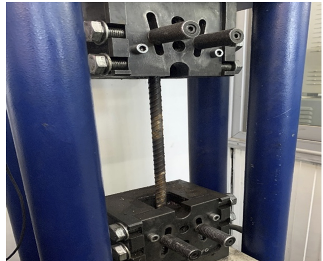
Fig. 2. Matest H010-02N uniaxial tensile strength device located at “ITM” laboratory
