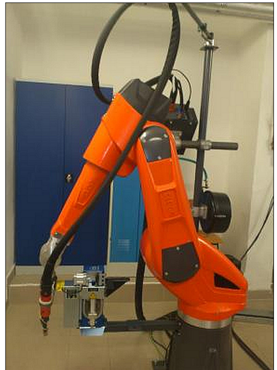
Figure 4. Cloos welder robot
