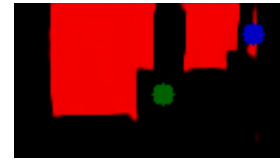
Fig. 5: Example for path search during flight. Green dot denotes pathway, which is considered free.
