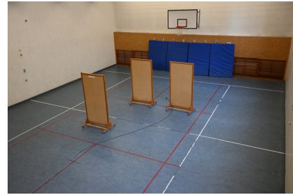
Fig. 9: Test track consisting of three display panels. The UAV had to avoid the front one, then pass through the two remaining panels.
