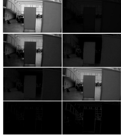
Fig. 1: Examples of the output images after processing: the six different contrast images [from up to down and left to right: rod image processing (grayscale image), amacrine image processing (grayscale image), blue cone image processing (blue color channel-based), red-green discrimination (red and green channel-based), yellow-blue discrimination (red, green and blue channel-based) and all cone discrimination (mean of all color channels)] and two examples from the 20 separate images containing edge-information.
