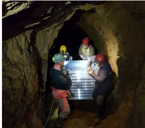
Figure 1: Transportation of the Large Muograph inside a tunnel in the Esztramos cave system.
