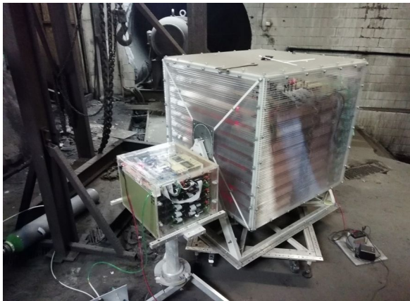
Figure 2: Small (25 cm) and large (80 cm) muographs next to each other in a tunnel underneath the Castle of Buda in Budapest.
