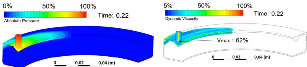
Fig. 5 Absolute pressure distribution (left) and oil spread with dynamic viscosity and maximal velocity (right) at normalized time of 0.22
