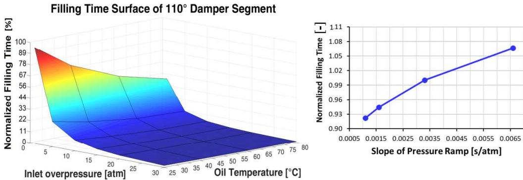
Fig. 7 Parameter sensitivity analysis of the inlet overpressure, oil temperature (left) and the slope of pressure ramp (right) on the filling time
