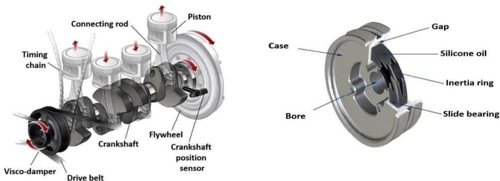
Fig. 1 Crankshaft configuration (left) and structure of a visco-damper (right) [8]
