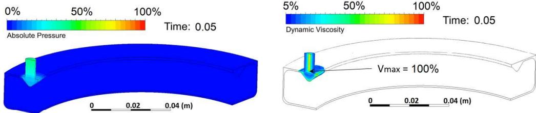
Fig. 4 Absolute pressure distribution (left) and oil spread with dynamic viscosity and maximal velocity (right) at normalized time of 0.05
