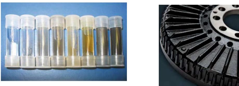
Fig. 2 Degradation levels in silicone oil samples (left) and cooling fins on visco-damper (right) [10] [9]
