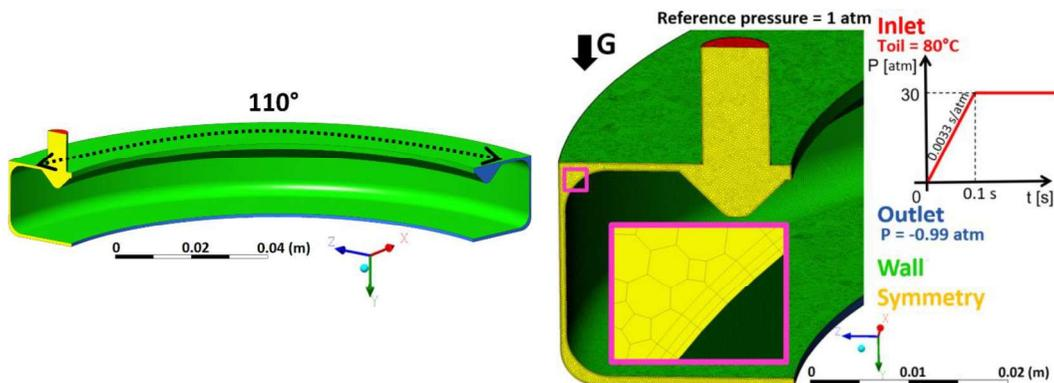
Fig. 3 The investigated flow field (left) with the numerical mesh, reference pressure, coordinate system, ruler and boundary conditions (right)
