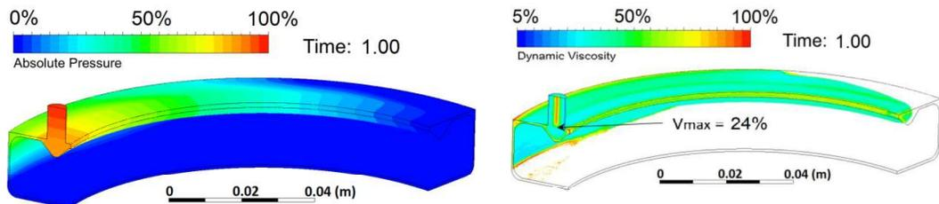
Fig. 6 Absolute pressure distribution (left) and oil spread with dynamic viscosity and maximal velocity (right) at normalized time of 1.00
