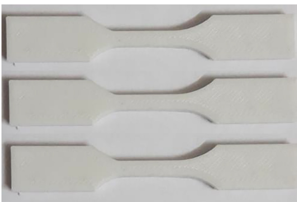
Fig. 4. The polylactic acid test specimens
