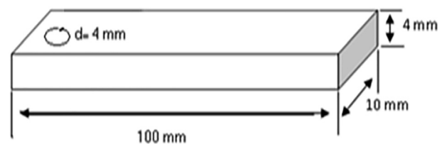
Fig. 5. Dimension of fatigue sample
