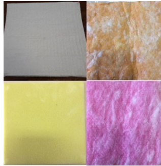
Figure 2. The tested materials (slentex, microfiber orange, polymeric, microfiber pink)
