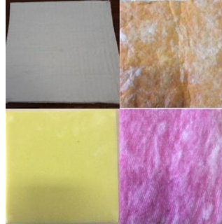
Figure 2. The tested materials (slentex, microfiber orange, polymeric, microfiber pink)
