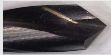
Implementation of macro groove on the rake face standard twist drill
