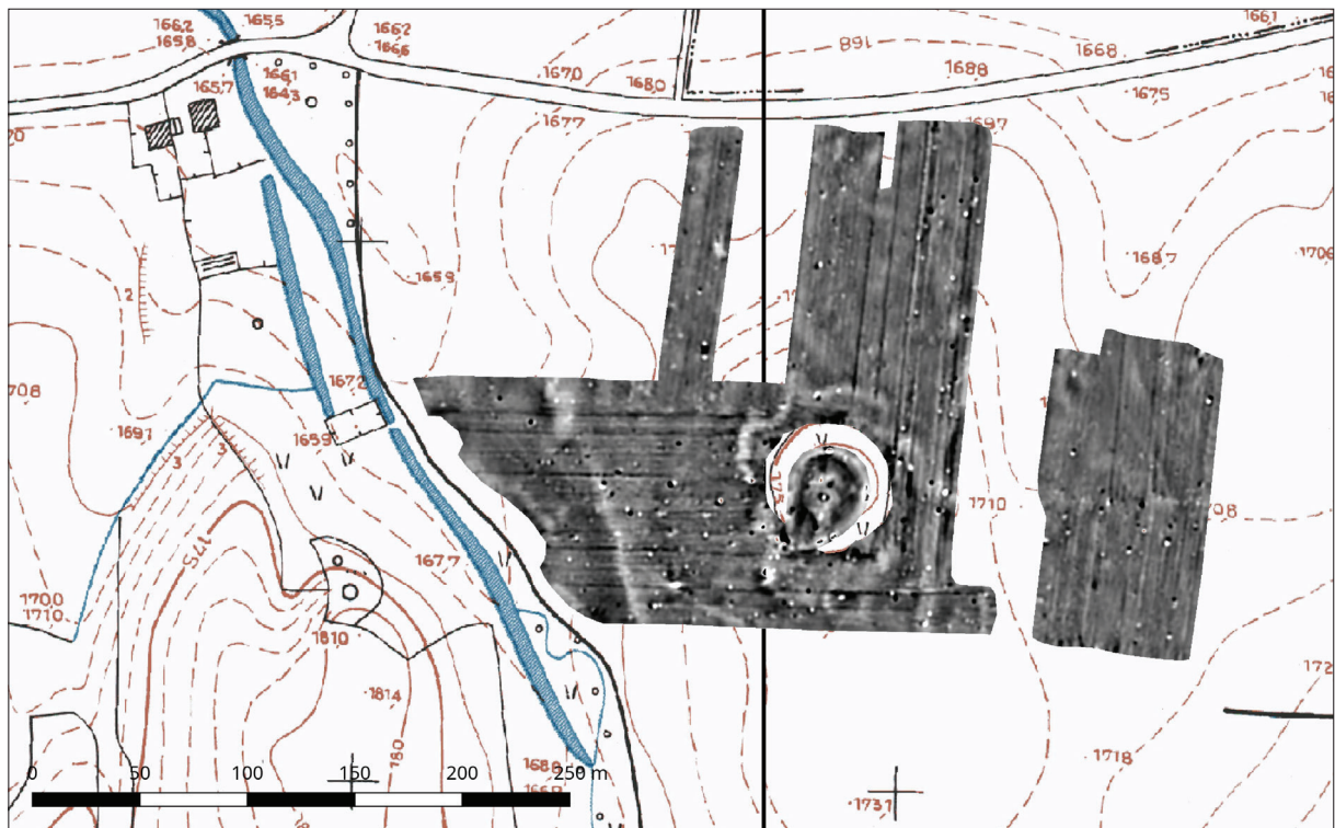
Fig. 12. Magnetic anomaly map in Jalžabet – Bistričak (Podravina, Croatia) implanted in Croatian base map 1:5000 (A. Bődöcs).
