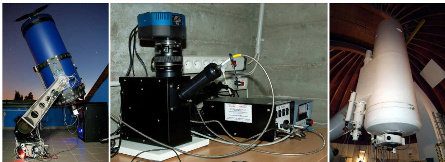
Figure 1. Left: The 0.5m RC telescope of GAO used exclusively for spectroscopic observations. Center: The eShell echelle spectrograph and its accessories: the QSI 532ws CCD camera and the ThAr unit with its power supply box in a thermally isolated concrete room below the 0.5m RC telescope at GAO. Right: 1m RCC telescope of PO.
