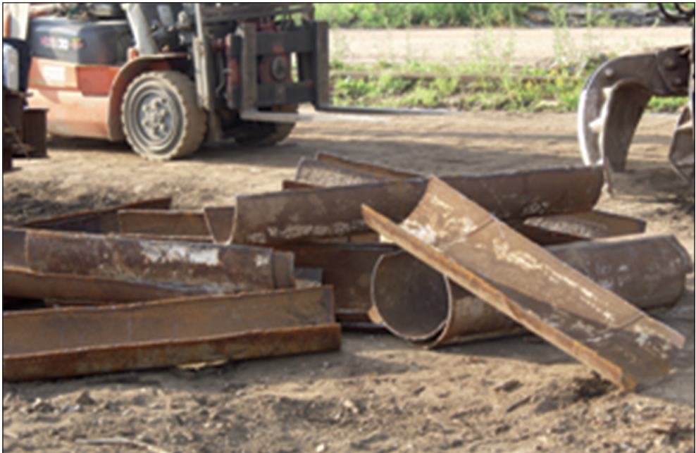
Figure 6: TENORM polluted steel pipes [14]
