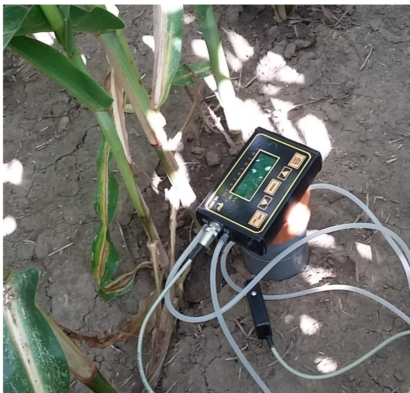
Figure 1: Measurement of CO 2 emissions at grain maize
