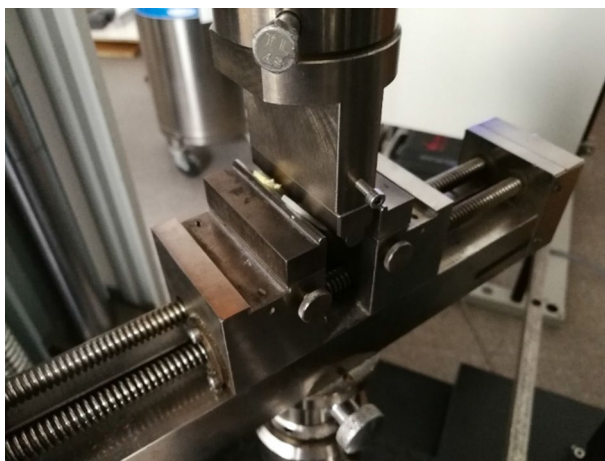
Fig. 1 The measurement setup for the free recovery experiments
