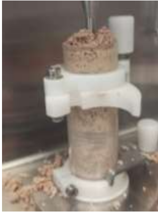
Fig. 4. Sample holder of SE testing.
