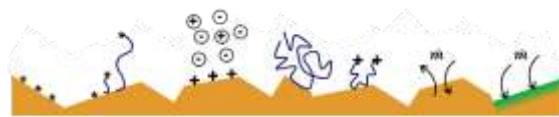
Fig. 3: Mechano-chemical effects at interfaces (from left to right): Radical formation, surface charges and double layers, adsorption, mass transport to and from the surface (incl. dissolution and uptake of solvents).
