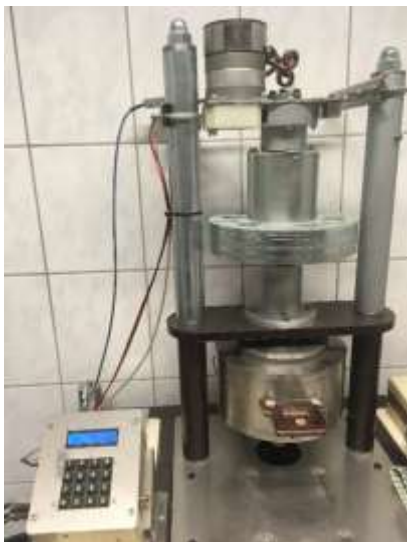
Fig. 2. Photo of the upgraded Universal Hardgrove mill.
