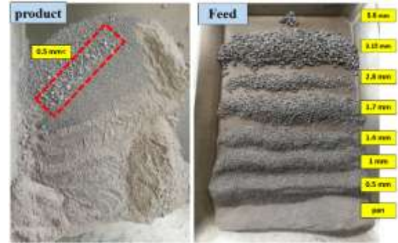
Fig. 4. Images of feed and product of the vibrating mill after sizing
