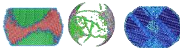
Fig.1: Phase transformation and defects observed in compressed nanoparticles by means of MD simulations (from left to right): Phase transition in ZnS (from wurtzite (red) to cubic (green) structure), dislocations in CaF 2 , shear planes in SnO 2 .
