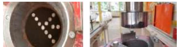
Fig. 2. Left: Die with pressure foils in one of the measurement layers; Right: piston after pressure application on wet material
