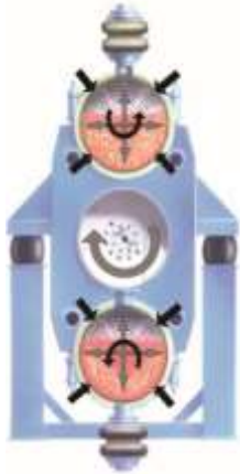
Fig. 1. Palla™ vibrating mill with charged grinding cylinders (Andres and Hude, 2010)
