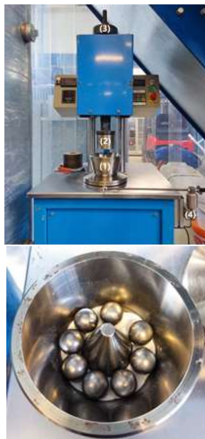
Fig. 1. Zeisel grindability device (up) and grinding bowl with balls and test powder (bottom). Grinding bowl (1), rotating die (2), disk weights (3) and load cell for torque measurement (4).
