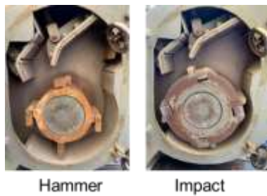
Fig. 2. Hammer rotor and impact rotor used in the mill
