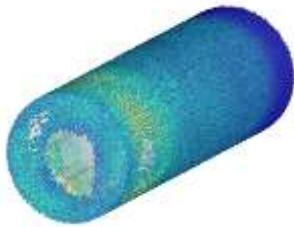
Fig. 1. CFD-DEM simulation of a wet-operated stirred media mill.
