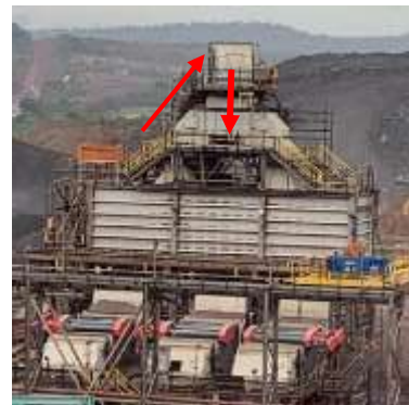
Figure 15. Example of parallel bin and screen placements – segregated material in bins due to the positioning of the conveyor drop angle.
