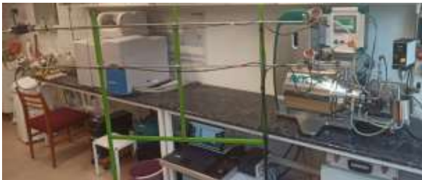
Fig. 3. Photo of the test rig with the on-line tube rheometer.
