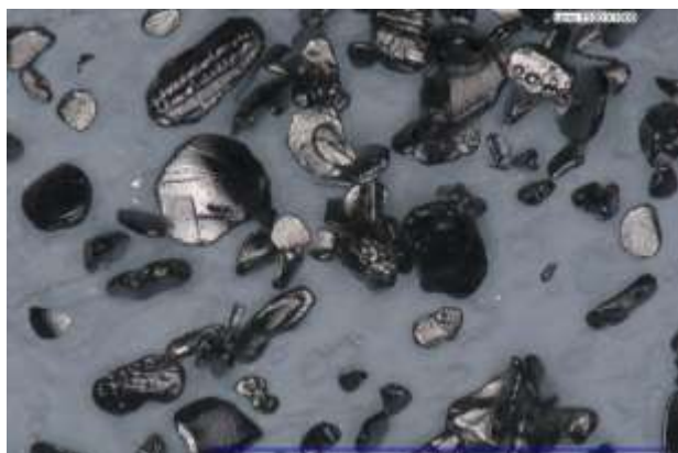
Figure 21: Synthetic graphite precursor; green/calcined coke
