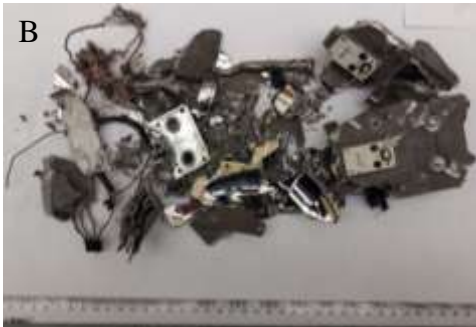
Fig. 8. Manually disassembled part (A) and product of hammer shredder (without screen) (B)
