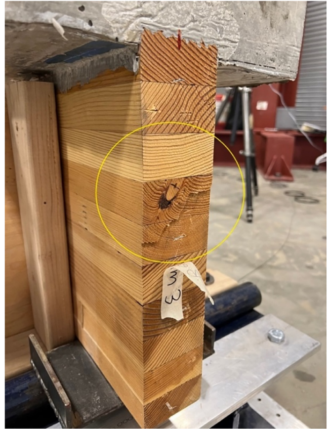
Fig. 7. Shear failure mode (S3)
