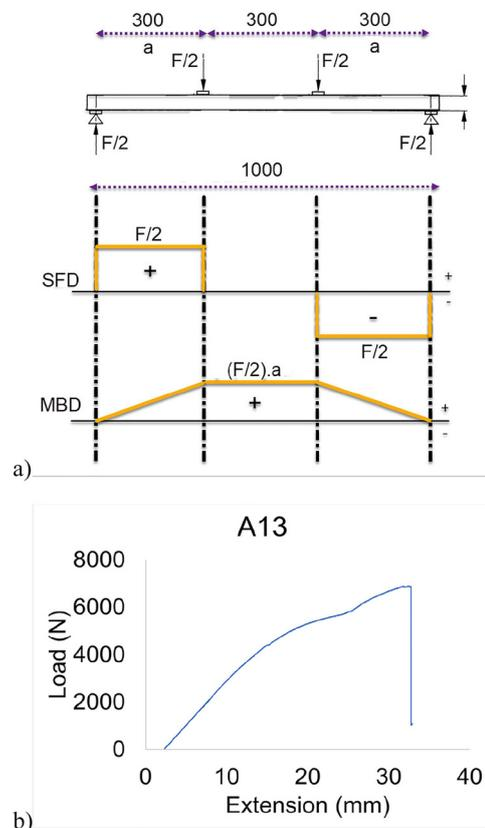
Fig. 1. a) Load analysis of the testing sample; b) load vs. displacement curve generated by the testing machine for sample A13
