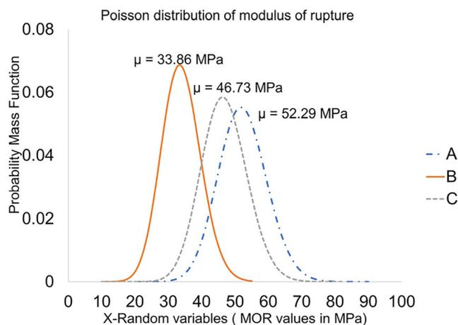
Fig. 6. Modulus of rupture representation in terms of Poisson's distribution
