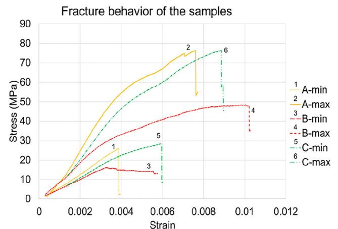
Fig. 3. Stress vs. strain diagram for maximum and minimum strength of rupture of tested groups
