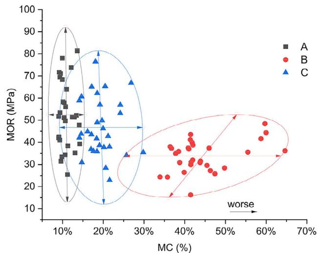
Fig. 5. MOR vs. MC 95% confidence ellipse graphs for the three groups of tested samples
