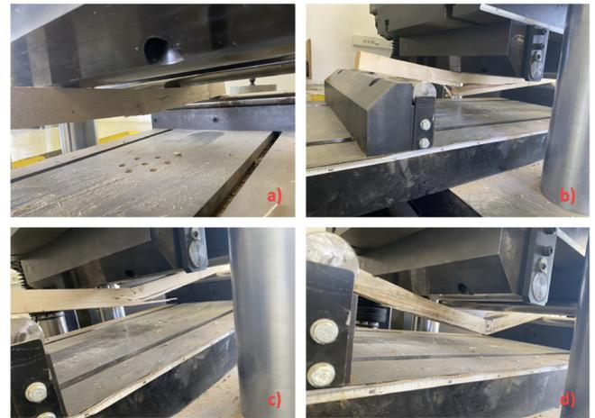
Fig. 2. Failure modes found during the test for the case of group A, a) simple tension failure; b) cross-grained tension failure; c) brash tension failure; d) buckling failure
