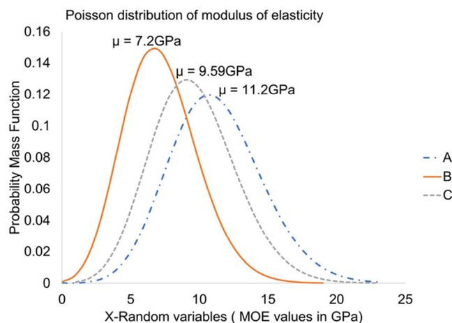
Fig. 7. Modulus of elasticity representation in terms of Poisson's distribution
