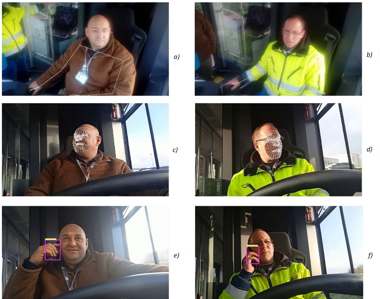
Figure 3 Monitoring results: a)–b) Pose estimation (preliminary results) for manual distraction detection; c)–d) Face and gaze detection for visual attention detection; e)–f) Mobile phone detection for distraction detection
