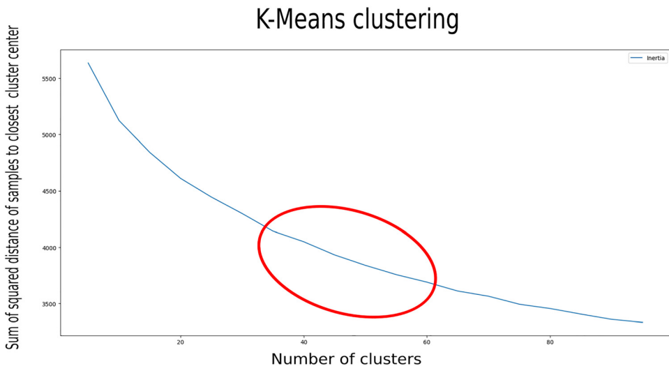
Fig. 2. Estimation of the ideal number of clusters in the whole labour law dataset. The X-axis shows the number of clusters, while the Y-axis shows the summary of the squared distance of the documents to the closest centroid. The squared distance is a calculation between each document and the centre of the topics of the given document. The ideal point and the ideal cluster value is the point of inflection of the curve ('the elbow'), where the graph starts to look like a straight line
