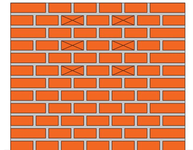
Fig. 1. Illustration about the masonry wall elevation view (voids are marked with X)
