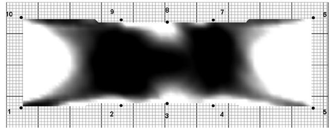
Fig. 3. Section view of the masonry wall plotted using ArborSonic3D (non-solid section)
