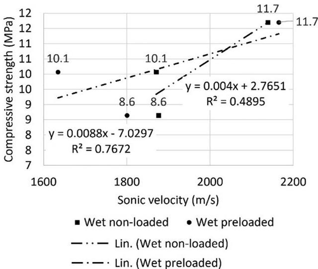
Fig. 9. Correlation between compressive strength of bricks and sonic velocities, wet condition
