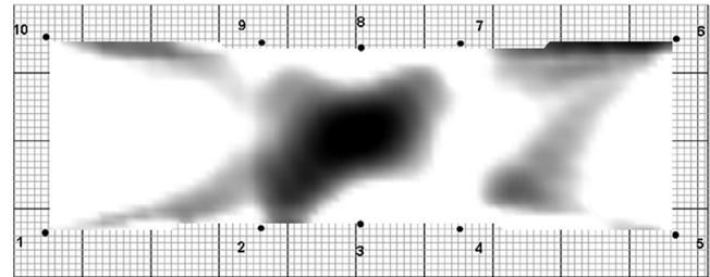
Fig. 4. Section view of the masonry wall plotted using ArborSonic3D (solid section)
