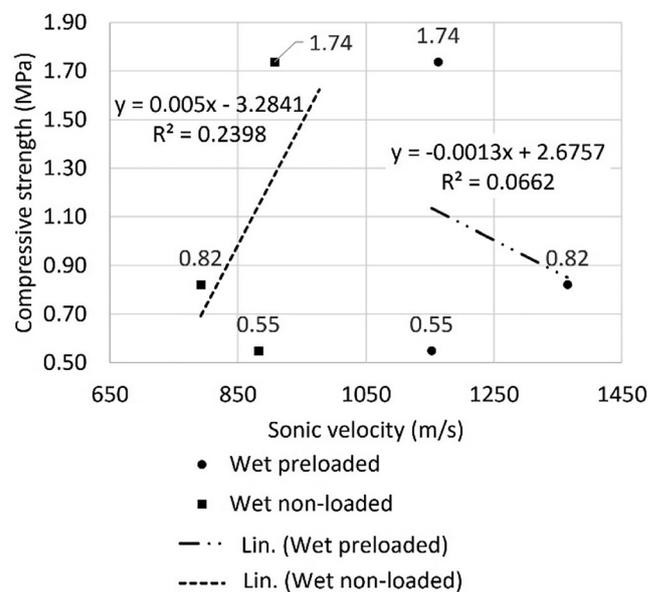
Fig. 7. Correlation between sonic velocity and compressive strength of mortars in wet condition
