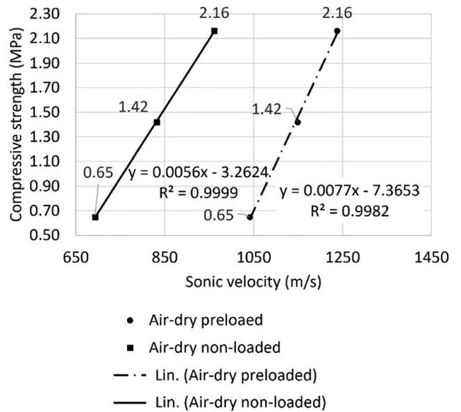
Fig. 6. Correlation between sonic velocity and compressive strength of mortars in air-dry condition
