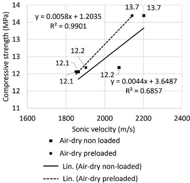
Fig. 8. Correlation between compressive strength of bricks and sonic velocities, air-dry condition
