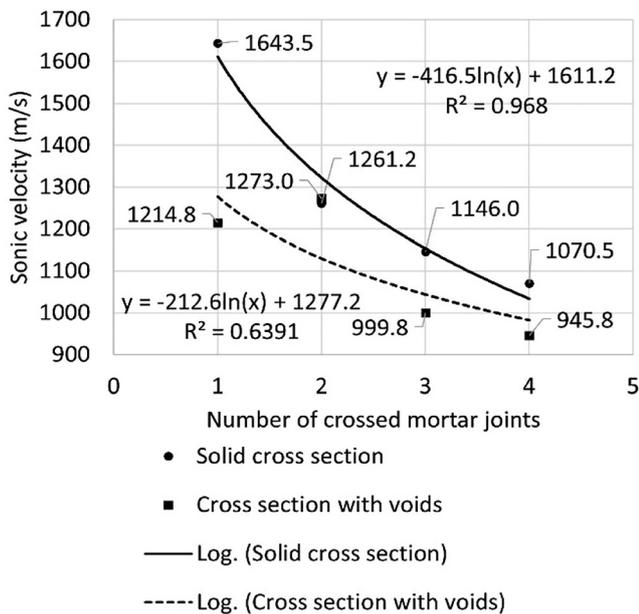
Fig. 5. Sonic velocities depending on the number of crossed joints
