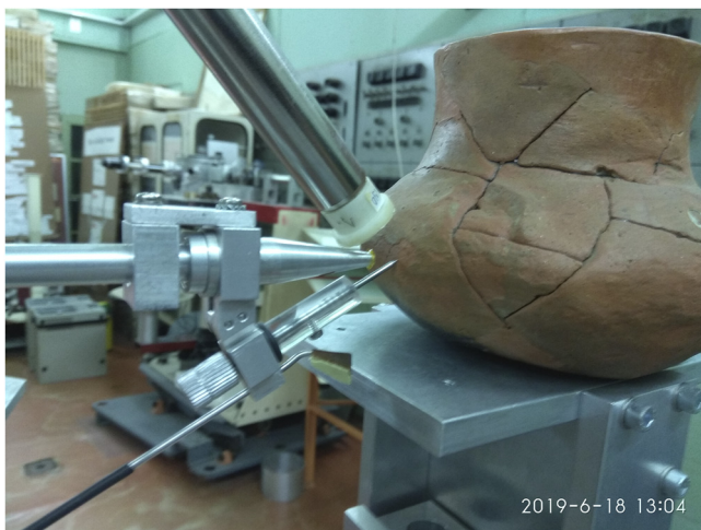
Fig. 3. The PIXE measurement setup for the mug from Nagykanizsa-Bilkei-dűlő. The pointer shows the examined surface
