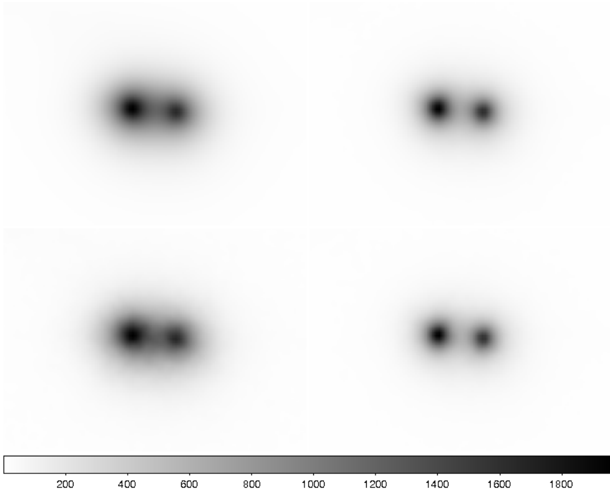
Fig. 2 Comparison of CE Cas with (right) and without (left) lucky imaging technique. Top left panel: sum of all the images only with tip-tilt correction, bottom left panel: sum of 300 randomly selected images, top right panel: sum of the best 750 (5%) frames, bottom right panel: sum of the best 300 (2%) images.
