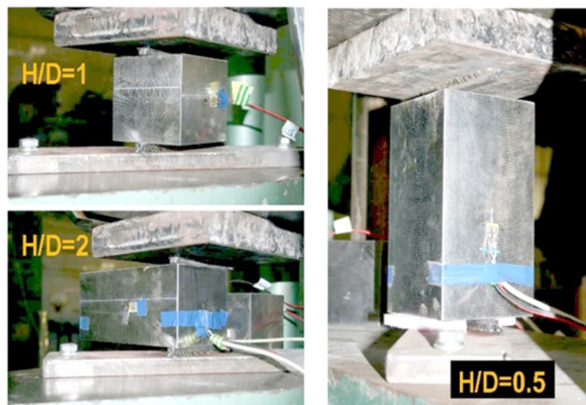
Figure 4. The tested steel specimens between the loading plates
