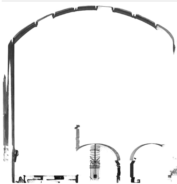
Figure 11. Elliptical-shaped diagonal section of the nave of the Franciscan Church of Szeged-Alsóváros
