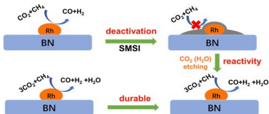
Fig. 56. Rh/BN catalyst deactivated after dry reforming of methane could be removed by CO_2 or H_2O treatment. Reproduced from Ref. [347] Graphical abstract.
