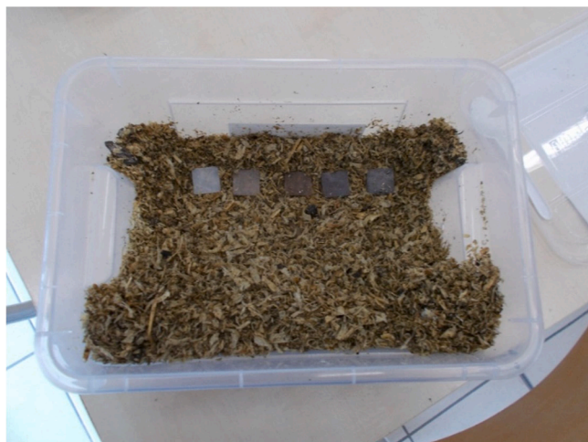
Fig. 1. A reactor with the composite specimens placed in it before being buried in the compost.
