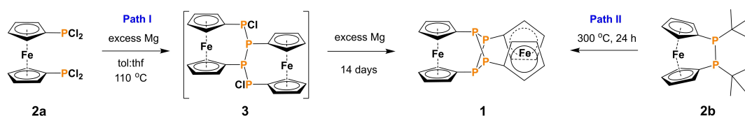
Scheme 1. Synthetic approaches to tetracyclic oligophosphane 1 .
