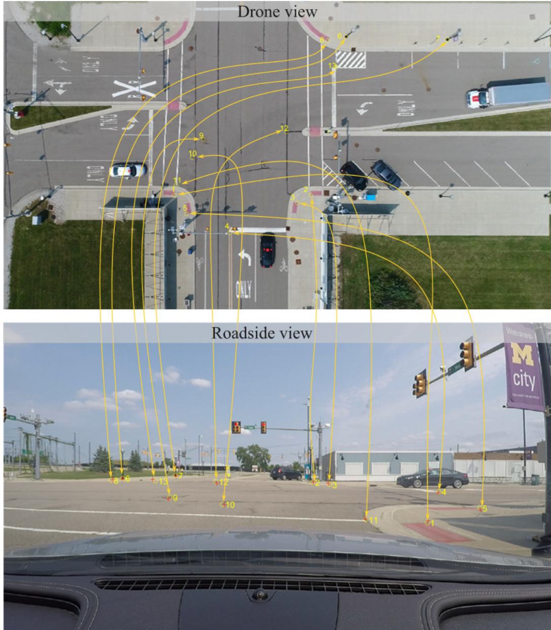
Figure 8. Points selected to map the drone view (upper figure) to the roadside view (lower figure). Yellow circles are hand selected points, and red crosses are calculated from the drone view points using matrix \mathbf{H} for validation purpose.
