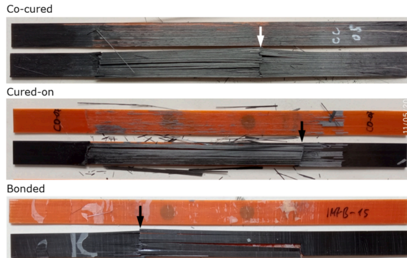
Fig. 10. Sandwich coupons opened after CF/EP fracture with arrows showing the CF/EP layer tensile failure locations. The CF/EP layer is attached to the lower part of all three coupons depicted.
